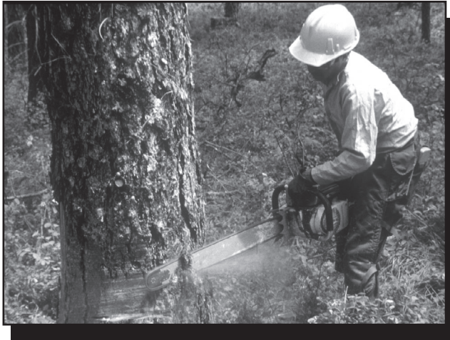
Figure 4-22—Bark can be removed with the tip of the bar.
