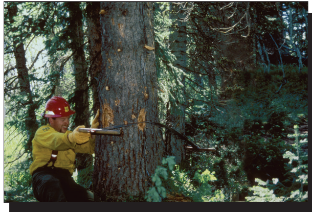
Figure 5-29—Gunning the saw helps determine the specific direction of the undercut. (Photo has been digitally altered to remove distracting items.)
