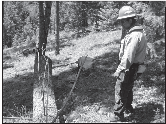
Figure 5-20—Determine the offside (usually the downhill side) and stay clear of that side when you are single bucking.
