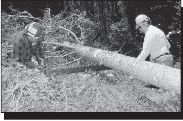
Figure 5-21—Watch the kerf for movement that will indicate a bottom bind (kerf opens) or top bind (kerf closes).
