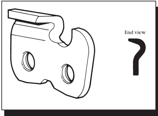
Figure 3-2—The chipper is the most versatile cutter type. Chipper chain is easy to file, will tolerate the most dirt, and can be used for many types of sawing operations.—Oregon Maintenance and Safety Manual, permission by Blount, Inc.
