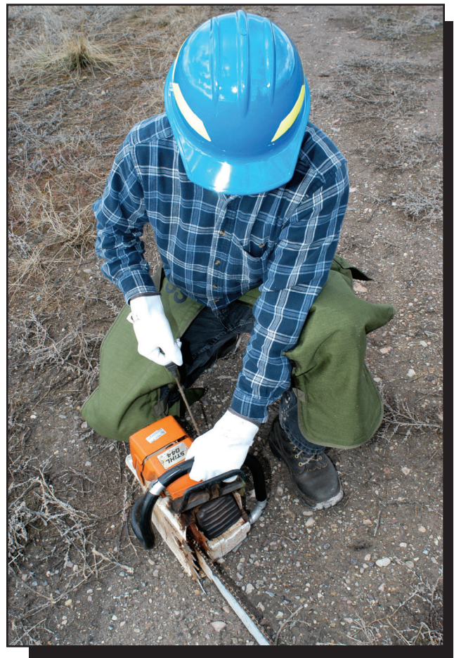
Figure 3-17—Start the saw on firm ground.
