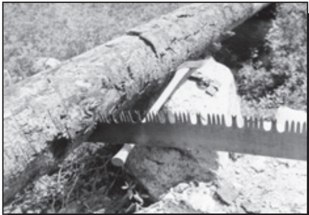
Figure 5-23—An ax planted in the lower part of the log can work as an underbuck.
