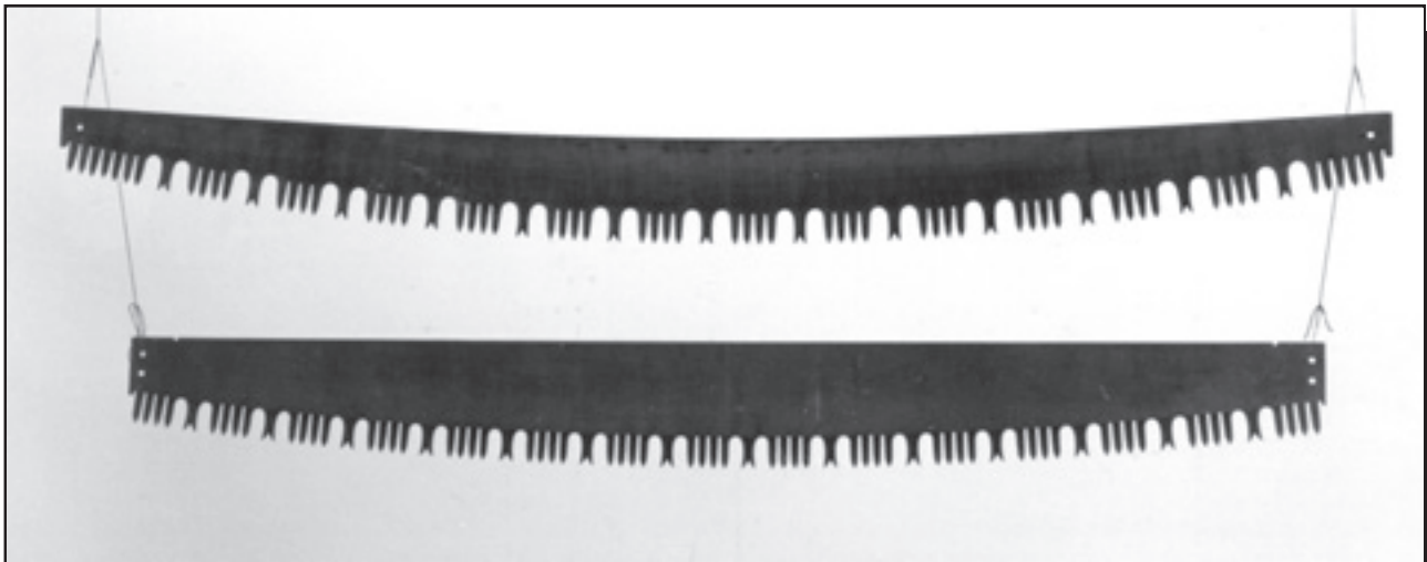
Figure 5-3—Comparison of felling and bucking saws. Concave-backed felling saws often have one handle hole per side. Straight-backed bucking saws can have two handle holes per side.
