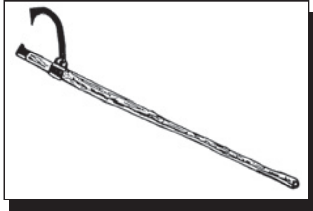
Figure 3-23b—The cant hook has a tow or lip at the lower end instead of a pointed spike like the peavey.
