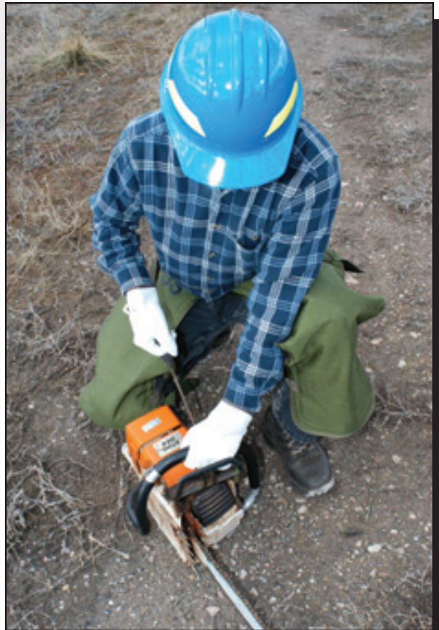
Figure 3-17—Start the saw on firm ground.
