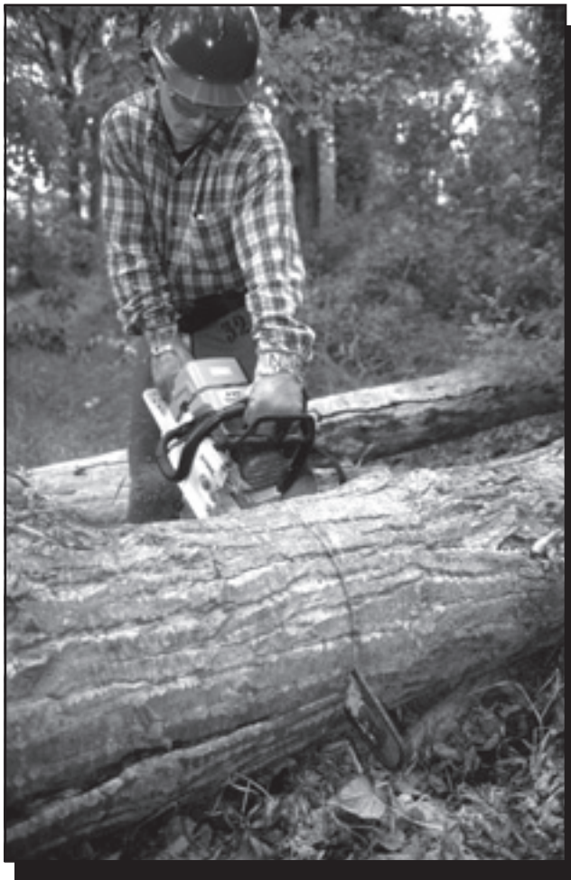
Figure 4-11—Watch the kerf for movement that will indicate a bottom bind (kerf opens) or top bind (kerf closes).
