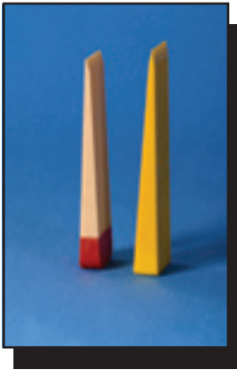
Figure 3-22—Double-taper wedges are designed to reduce bind.
