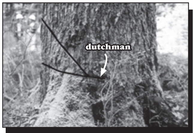
Figure 4-24—When the sloping cut and the horizontal cut do not meet exactly, a dutchman is formed. This kerf-wide cut makes the direction of the tree's fall harder to predict. It can also cause the tree to barber chair, lifting the log off the stump and placing the sawyer at great risk.
