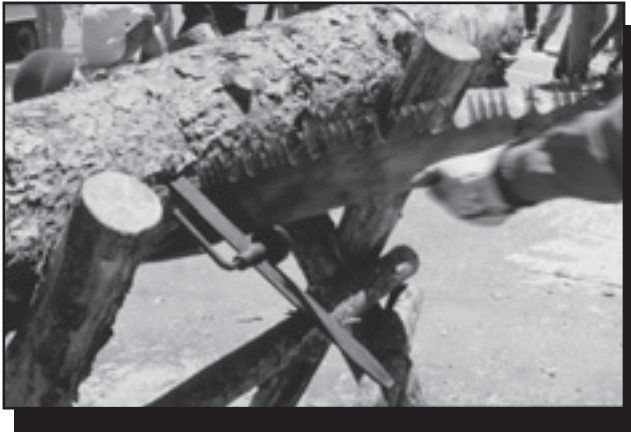
Figure 5-15—A mechanical underbuck helps hold the saw up when cutting from the underside of the log.
