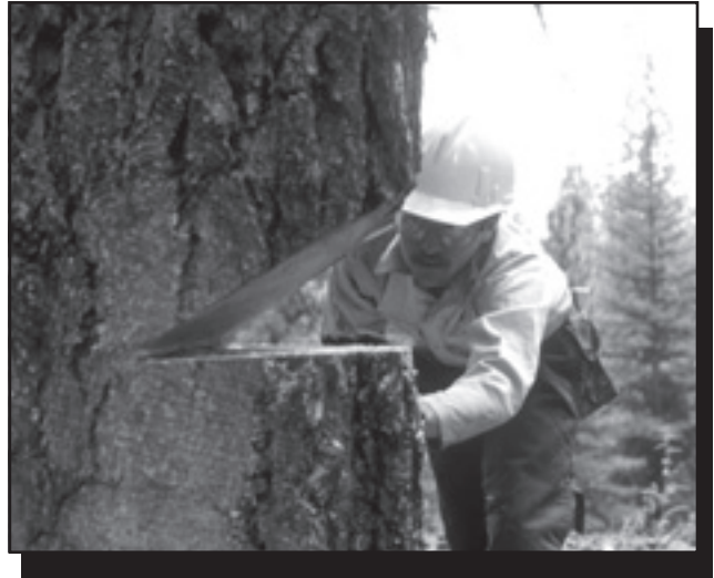
Figure 4-23—The sloping cut is a 45-degree angle.
