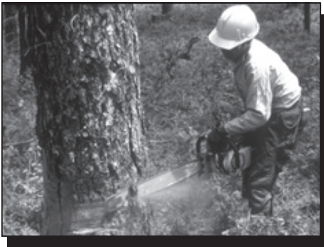
Figure 4-22—Bark can be removed with the tip of the bar.
